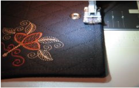
22. Top stitch around case with accurate 1/4" seam.
