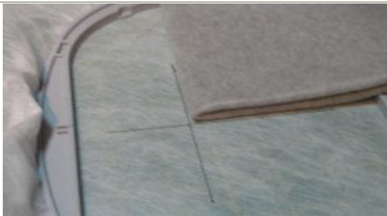
5 – Place folded fabric inside corner of placement lines. Unfold fabric flat, secure with temporary adhesive spray. (3" marked line should be on right side facing vilene).
