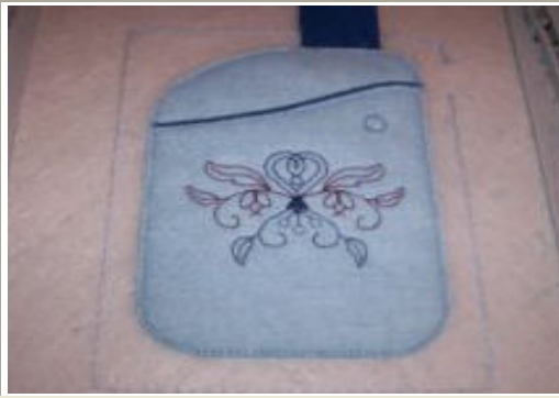
18. Remove hoop, trim fabric around pocket close to outline. Put hoop on machine.
