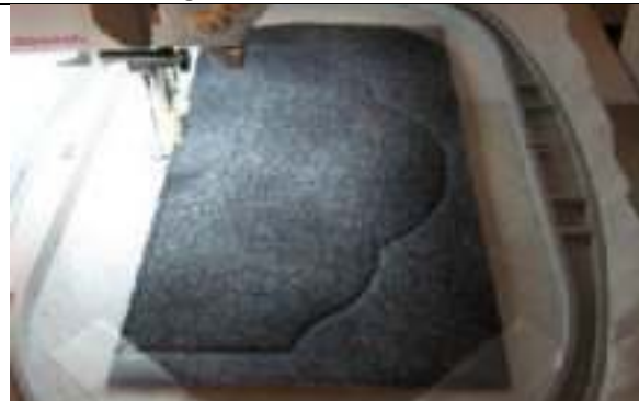
4. Put hoop on machine. The 2 nd color in the design tacks the fabric & fleece down. (also top stitches turned/folded edge on the left side)
