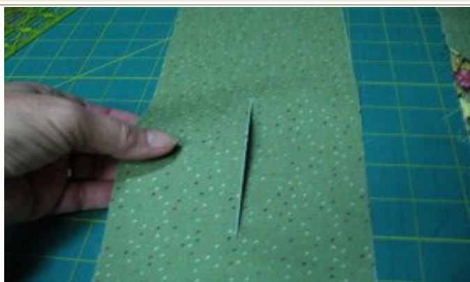
19. On lining (back) pieces. Measure up 2" from the bottom, mark line 7"-8" long centered. Cut marked line open with ruler & rotary cutter (both pieces).
