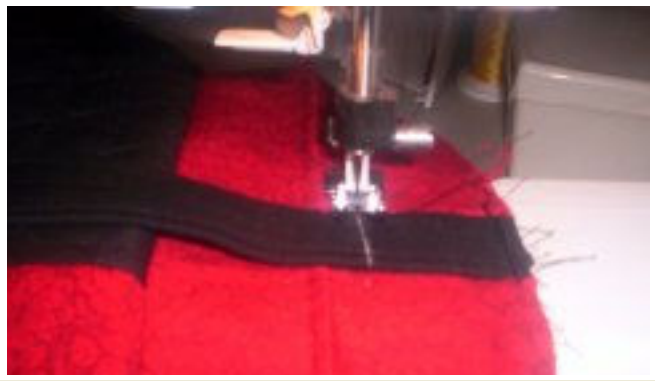
21. Stitch straps to purse at top with 1/4" seam & then top stitch twice over 1 1/2" marks on each strap to secure.
